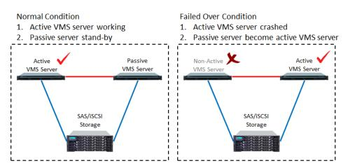
In our real test, the SAS storage would take 2 minutes to finish the failed-over transition. And the iSCSI would like 6 minutes.
