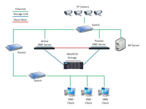
In the normal condition, the active VMS server will service and the passive VMS server will standby. Besides, our VMS server is equipped with watchdog to prevent software level crash. Once the active server encounter the hardware level fatal case, Microsoft cluster will wake up the passive VMS server and the passive VMS server will change to active one.
